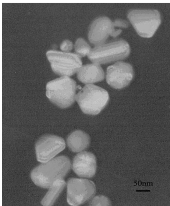
Figure 1 Typical TEM micrograph of the silver nanoparticles prepared by sodium citrate reduction of \text{AgNO}_3 .
